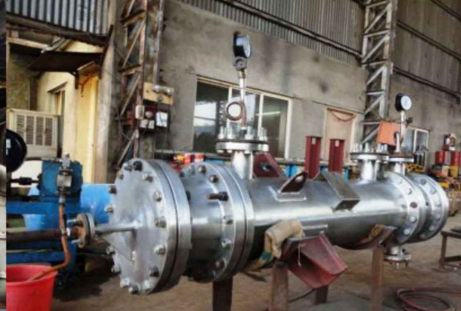
SIDE STREAM FILTER VESSEL - HPCL RAJASTHAN REFINERY PROJECTS WEIGHT - 43 MT, DIA. 3400 X 11000 MM LOS.
