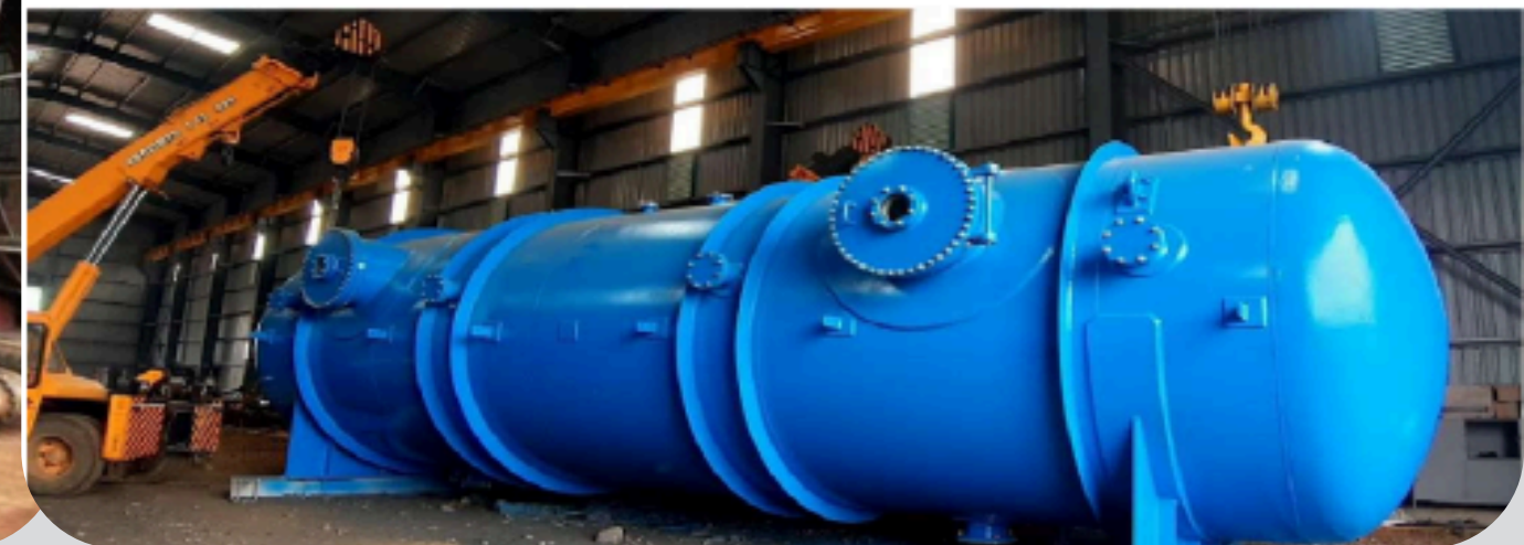
SIDE STREAM FILTER VESSEL - HPCL RAJASTHAN REFINERY PROJECTS WEIGHT - 43 MT, DIA. 3400 X 11000 MM LOS.
